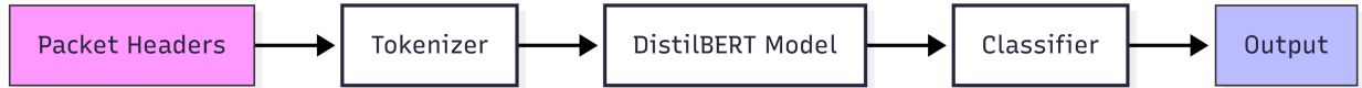
Figure 1: The system architecture, showing the flow from packet headers to classification output.
